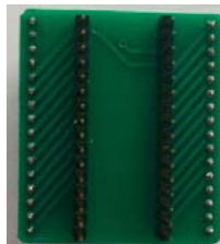
Transition Socket of LQFP32 (back)
