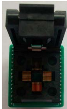
Transition Socket of LQFP32 (front)
