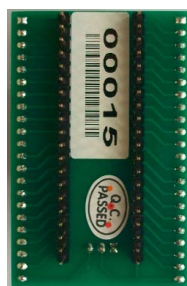
Transition Socket of LQFP44(back)
