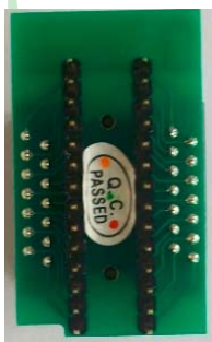
Transition Socket of SOP28 or SOP20 (back)
