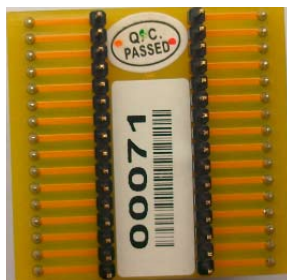
Transition Socket of SOP32 (back)
