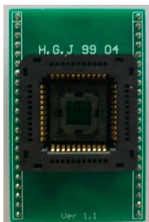
Transition Socket of PLCC44(front)
