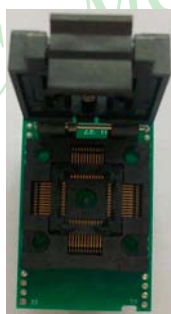
Transition Socket of LQFP44(inside)
