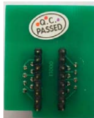
Transition Socket of SOP16 or SOP8 (back)
