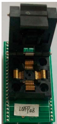
Transition Socket of LQFP48(inside)
