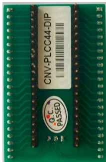
Transition Socket of PLCC44(back)
