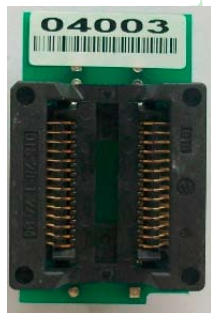
Transition Socket of SOP28 or SOP20 (front)
