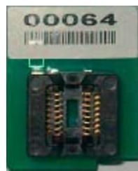
Transition Socket of SOP16 or SOP8 (front)
